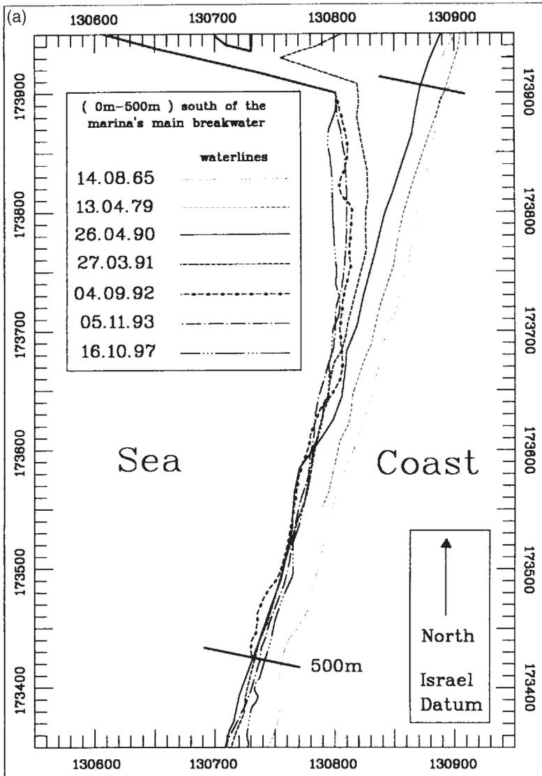
Fig. 3. (a) The waterline as shown on aerial photographs (1965–97) for the first 500 m of coast south of the marina's main breakwater.
