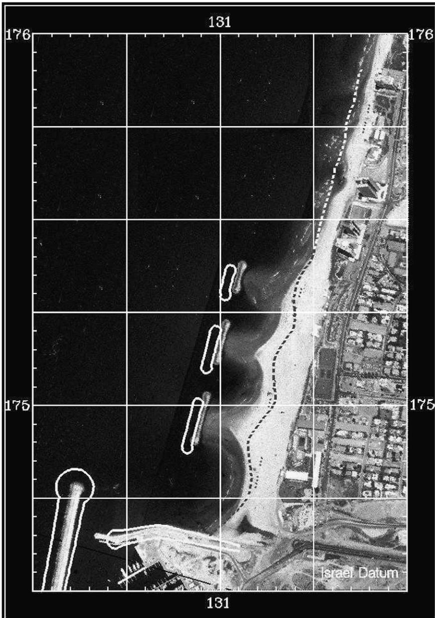
Fig. 2. The predicted shoreline for the option C sedimentological balance (dotted line) superimposed on background aerial photograph No. ML/538 (8 June 1996) showing the observed waterline.
