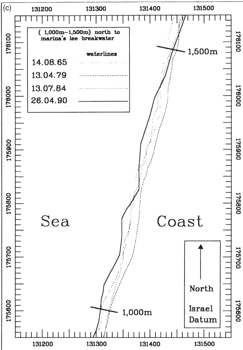
Fig. 3. (c) The waterline as shown on aerial photographs (1965–90) for the coastal segment 1000–1500 m north of the marina's lee breakwater.
